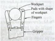
Figure 4. Single or Double type Gripper
