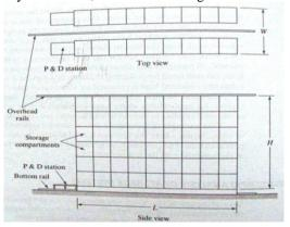
Figure 5. Sizing AS/ RS Rack Structure
