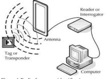
Figure 1:Radio frequency identification system
