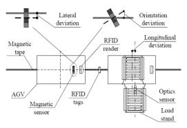
Figure 2. AGV docking process
